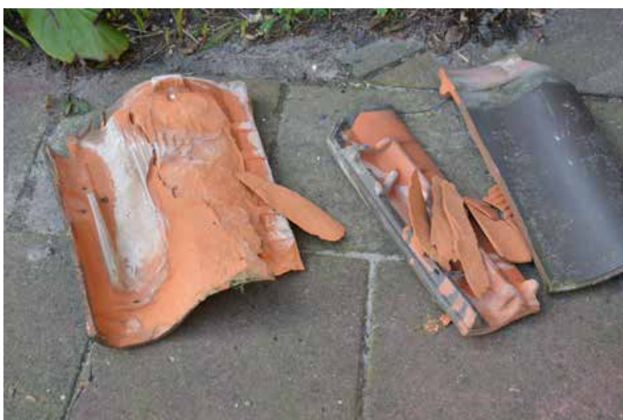
Figure 5.2a/b A more urgent problem: several tiles show frost damage, causing leakage, with consequential danger for the underlying timber construction
